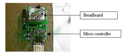
Figure 6 – Micro Controller with breadboard and ULN2803A, LEDs, wires leading to robot.
