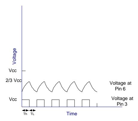
Figure 5 – The timing of the signal in the controller circuit
