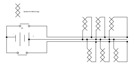
Figure 3 – The manual controller shown is wired for a pace gate.
