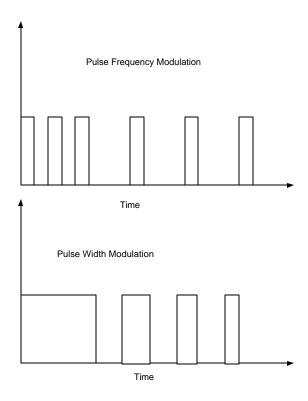
Figure 6 – The idea of PFM and PWM. PFM keeps the pulse width constant and varies the time between pulses and PWM keeps the time between pulses constant and varies the pulse width.
