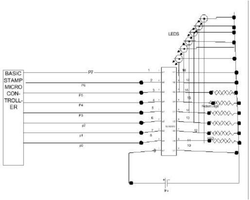
Figure 7 – The schematic of the micro controller. The ULN2803A chip is used again to drive the current to the robot legs. LEDs light up as the current is sent to the legs so we can observe the gate that the robot should be using by observing the LEDs. The program used to set the gates is listed in Appendix A.
